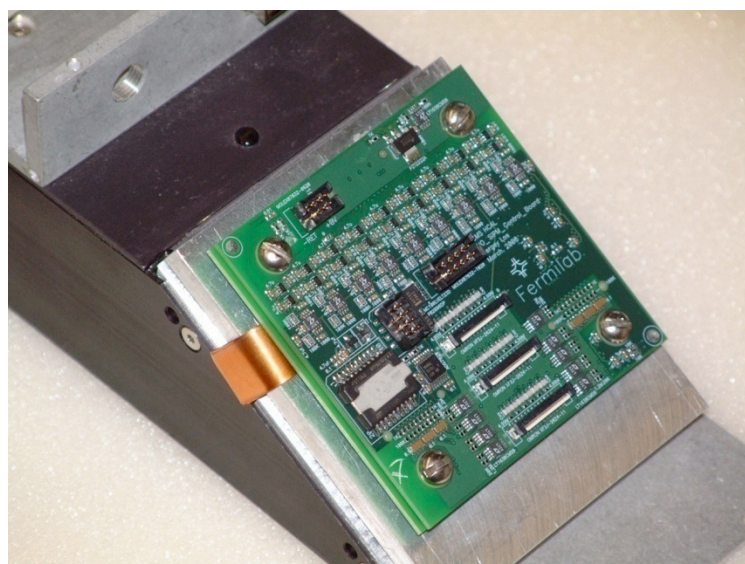
Figure 4.6: The Control Board. This board generates the SiPM bias voltages, measures the leakage currents, controls the Peltier cooler, and monitors voltages and temperatures.
